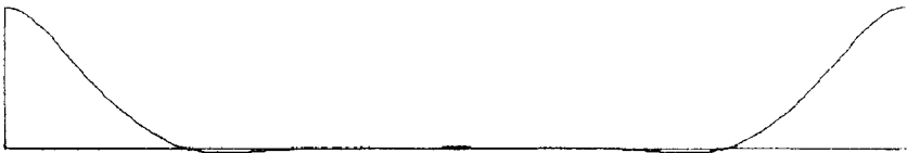
FIG. 3. The Lagrange function for analytic Poisson splines associated with g(t) = (1 - p^2) / (1 + p^2 - 2p \cos(t)) ( p = 1/2, n = 5 ) (see [3]).
